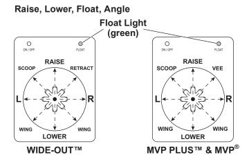
Moving the control lever in straight lines up and down or from side to side on the control body will result in the following blade movements:
