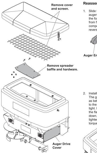
4. Remove the auger drive cover. Set the cover and all hardware aside. Remove all four bolts that hold the motor and gear box to the frame. Slide the motor and gear box out of the frame. Once the gear box is removed, the auger can be removed.
