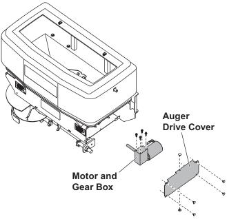
3. Position the auger so that the auger and auger tube sit unobstructed in the hopper tub. Once the tube is positioned, mark the mounting holes on the auger gear box side position.
