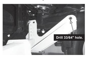
Locate the 1/2" x 1-1/4" cap screws with 18" handles. Insert the cap screws with handles into the frame and out through the holes drilled in Step 6. Install 1/2" locknuts on the cap screws and finger tighten.
