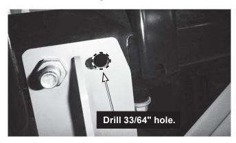
9. Place 1/2" washers on the 1/2" x 1-1/2" cap screws with 7" handles. From inside the frame, install the cap screws through the holes drilled in Step 8. Install 1/2" washers and 1/2" locknuts on the cap screws and finger tighten.
