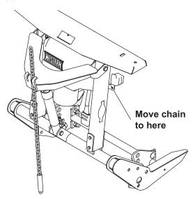
2. Remove and retain the two hairpin cotters, washers and pins attaching the lift arm to the lift frame.
