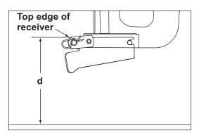
2. Use dimension "d" from Step 1 and the following chart to determine the proper pivot plate mounting position and pivot hole selection.
