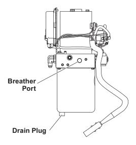
6. Install the 90° elbow into the port, pointing up. Install the breather into the elbow.
