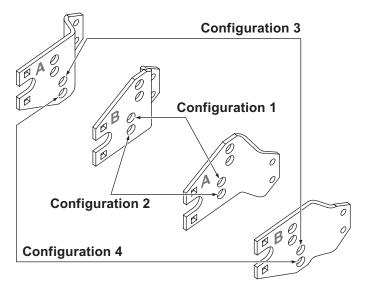
In each pivot plate mounting position, the pivot bar pins may be installed through either of the **lower** holes in the pivot plates, providing four different height adjustment positions. **The pivot bar pins are never installed in either of the two upper holes in the pivot plates.**
