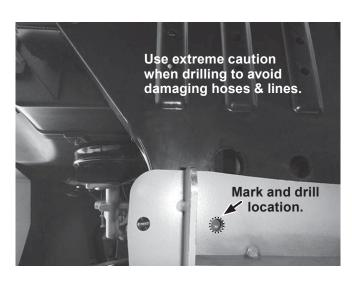
NOTE: Use extreme caution when drilling to avoid damage to hoses and lines located against the inner frame surface.
