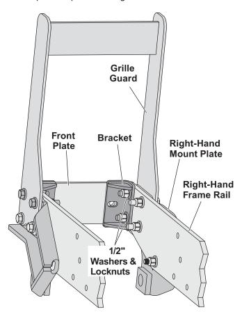
8. Place the front mount plate against the front frame plate of the tractor. Install two 1/2" x 2" cap screws through the holes of the mount plate and out through the brackets. Secure the cap screws to the brackets with 1/2" washers and 1/2" locknuts. Hand tighten.
