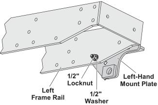
4. Position the grille guard over the left-hand mount plate. Place a 1/2" washer on each of two 1/2" x 2-1/2" cap screws\*. Align the holes in the grille guard, mount plate, and tractor frame. Install the cap screws with washers through the rearmost holes of the grille guard/mount plate/ frame. Secure the fasteners with 1/2" washers and 1/2" locknuts. Hand tighten.
