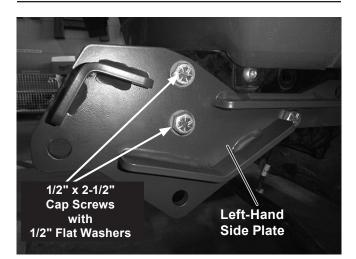
5. Install one 1/2" x 2" cap screw through the middle hole of the left-hand side plate as shown. Secure with a 1/2" washer and 1/2" locknut. Hand tighten.
