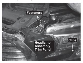
3. From the inner edge, release the headlamp assembly trim panel clips. Start at the outer edge of the assembly to release the headlamp assembly trim panel.
