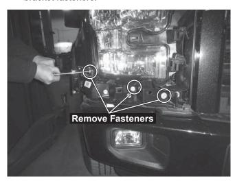
8. Squeeze the tabs with needle-nosed pliers to remove the headlamp assembly trim panel bracket.
