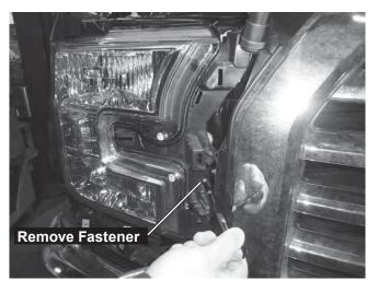
12. Position the headlamp assembly forward and disconnect the remaining electrical connectors.
