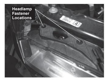
11. Remove the fastener on the side of the headlamp.
