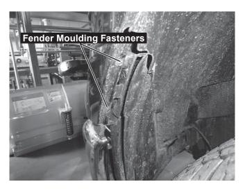
2. Release the three fender moulding locks and partially remove the fender moulding.
