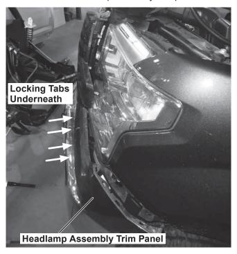
5. Remove the three fasteners on the headlamp trim panel bracket.
