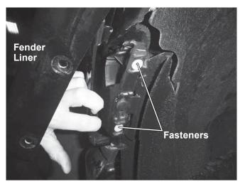
2. To remove the headlamp assembly trim panel, start by removing the fasteners shown.
