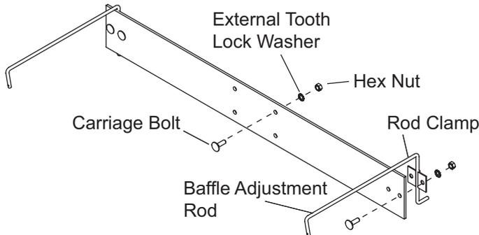
3. Place the assembled deflector on the spreader behind the spinner. The carriage bolts should be pointing toward the truck. Secure the deflector to the deflector plate with four 5/16" external tooth lock washers and four 5/16" nuts.
