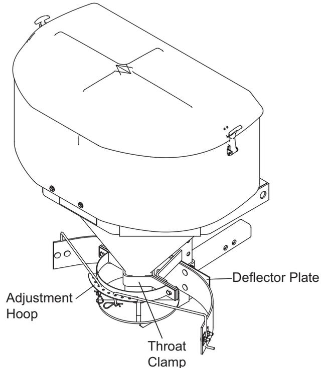
5. Insert the adjustment rods into the desired holes on the adjustment hoop and secure with the supplied hairpin cotters.
