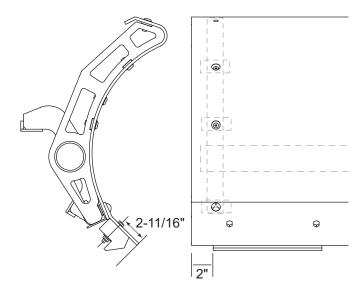
4. Mount shoe to desired height as shown in the following diagram. Shoe height is adjusted by mounting through the next higher set of holes. Secure with two 5/16" x 2-1/4" cap screws, 5/16" washers, and locknuts.
