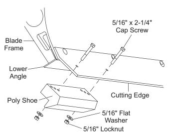
3. Using the lowest set of holes in the shoe as a guide, drill two 11/32" diameter holes on each end of the blade.
