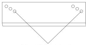
Drill two 11/32" dia. holes using these holes as a guide.
