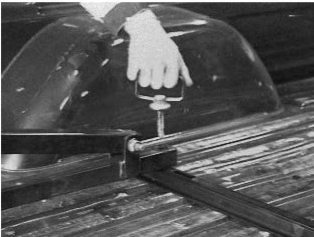
4. Center the mount assembly side to side in the vehicle bed. Verify trusses are perpendicular to the back angle.
