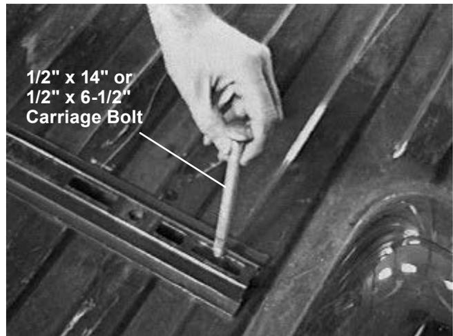
11. Secure the channel using one 1/2" top lock flange locknut on each side below the angle bracket. Verify the channel is still centered side-to-side in the vehicle bed and parallel with the back of the bed.
