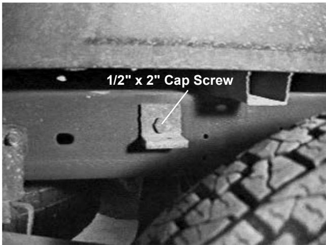
8. Insert bolts from the outside of the vehicle frame. Tighten according to the torque chart.
