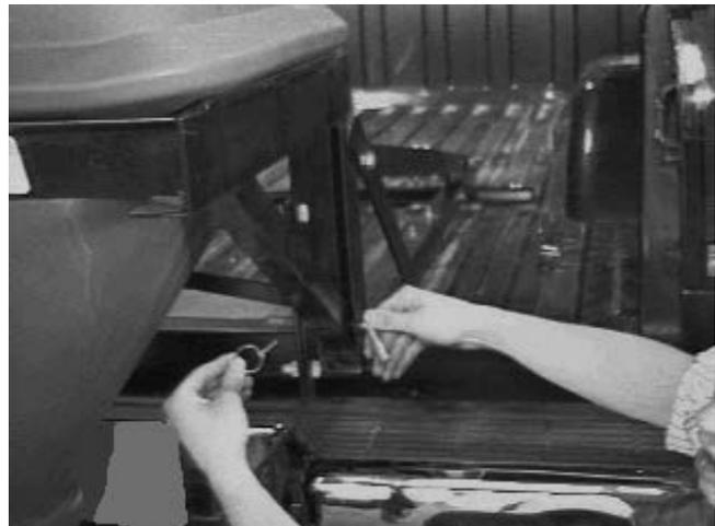
8. Connect spreader-side wiring harness to vehicle-side wiring harness.
