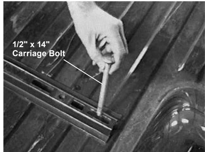
**NOTE: The carriage bolt on the outside of the vehicle frame should also pass through the wood block (if required).**
