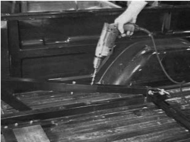
**NOTE: Pay special attention when drilling or clamping dissimilar metals to aluminum bodies. Galvanic corrosion can occur if not handled properly. Contact vehicle manufacturer for recommended attachment practices.**
