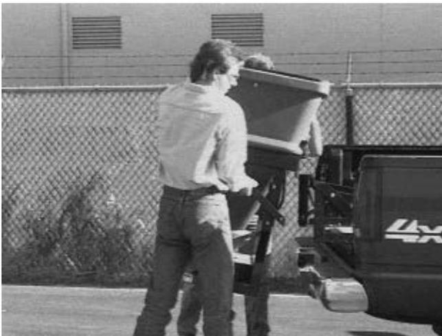
5. Position tabs on the spreader assembly over the top of the mount assembly and lower the hopper assembly.
