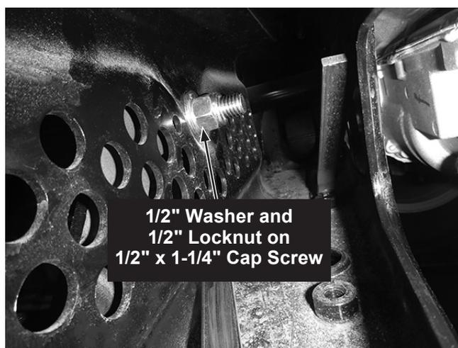
14. With the help of another person, reinstall the bumper. Trim the plastic air dam as necessary to install the mount beam between the passenger- and driver-side hanger assemblies. Insert 1/2" x 1-1/4" cap screws through the hanger assemblies and the mount beam (8 total). Secure each fastener with a 1/2" locknut. Hand tighten.
