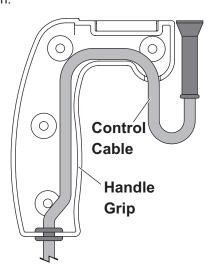
With the control cable in place, sandwich the handle grip halves around the pair of tabs corresponding to the desired handle alignment.
