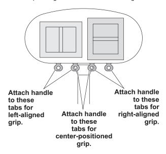
4. Secure the handle grip halves with the four socket head cap screws and four locknuts.
