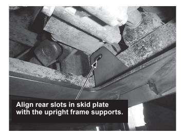
Place a 3/8" washer on each of two 3/8" x 1-1/4" cap screws. Install the fasteners through the holes in the upright frame supports. Secure the cap screws with 3/8" washers and 3/8" locknuts. Hand tighten.
