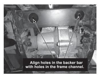
3. Use a floor jack to position the skid plate assembly against the bottom of the vehicle. Line up the middle slots of the skid plate assembly with the holes in the backer bar previously installed.
