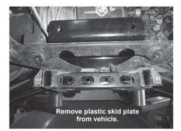
2. Place the backer bar inside the front frame channel with the holes in the bar aligned with the large holes in the frame channel as shown.
