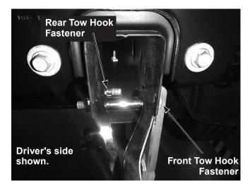
For models not equipped with tow hooks (2022 Mid-Year Refresh models): Place the driver-side mount against the outside of the driver-side frame rail. Install a 1/2" x 1-1/2" cap screw through the front hole of the mount. Secure with a 1/2" washer and 1/2" locknut. Hand tighten.
