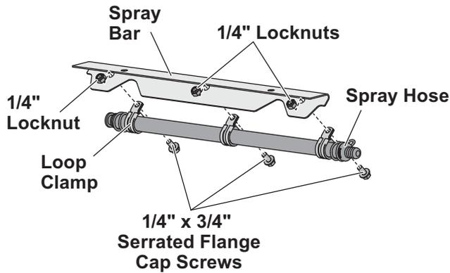
3. Use two 1/4" x 3/4" serrated flange cap screws with 1/4" locknuts to fasten the spray bar assembly to the sill extension cover as shown.
