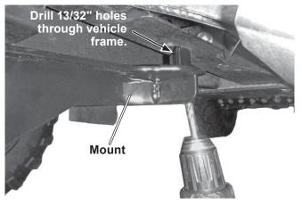
11. Place a 3/8" washer on a 3/8" x 2-1/2" cap screw and install it through the hole drilled in Step 10 and through the rear mount hole. Secure with a 3/8" locknut. Repeat for the opposite side.
