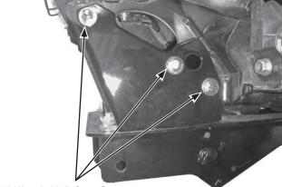
5/16" x 1-1/4" Cap Screws, 5/16" Washers, and 5/16" Locknuts
