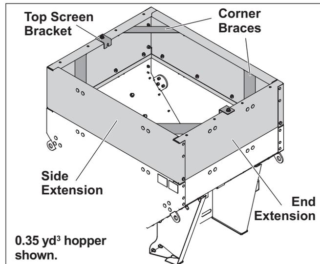
7. **For 0.35 yd<sup>3</sup> spreaders:** Reinstall the top screen and top screen brackets into the rivnuts on the top of the driver-side and passenger-side extension panels using two 3/8" x 1" serrated flange cap screws.
