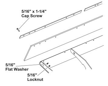
On 6' 8" blades, the deflector extends beyond the ends of the blade. Trim excess length from both ends of deflector and retainer bars as shown.
