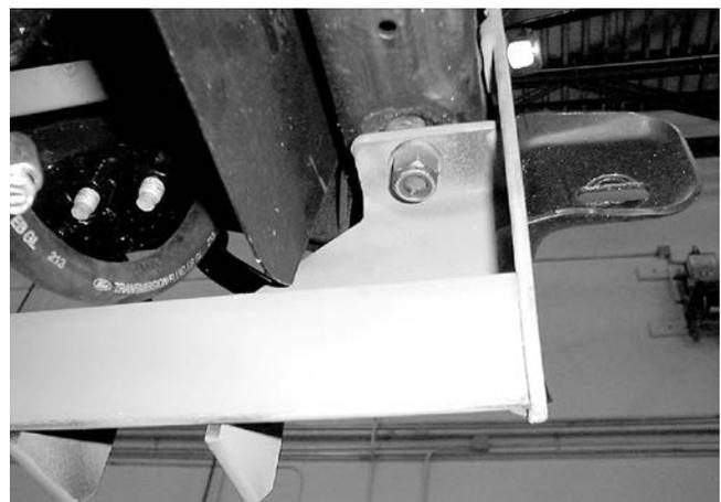
4. Push the front mount as far back as it will go, and tighten all four fasteners.
