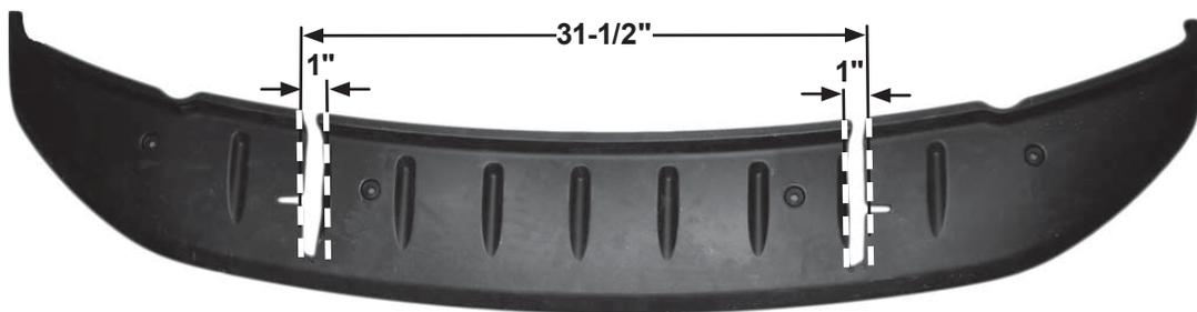
Cut slots in air dam as shown.
