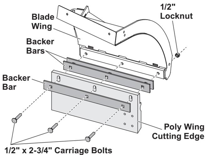
If keeping a steel cutting edge on the blade, use three 1/2" x 2" carriage bolts and no backer bars between the wing cutting edge and wing. Install the poly cutting edge using 1/2" x 2" carriage bolts instead of the 1/2" x 2-3/4" carriage bolts.
