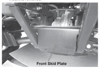
4. Remove the front skid plate. Retain for reinstallation if mount is removed.
