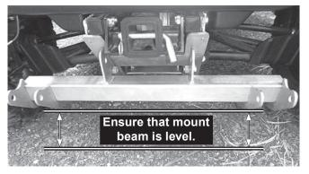
11. Measure the distance between the mount beam rear hole and the ground. If it exceeds 11-1/2", install the accessory Height Adapter Plate Kit (PN 77555) to ensure optimum plowing performance.
