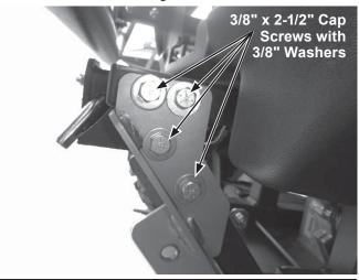
6. Place 3/8" washers on two 3/8" x 2-1/2" cap screws. Install the fasteners through the lower frame connection and the skid plate assembly. Secure with 3/8" washers and 3/8" locknuts; hand tighten.
