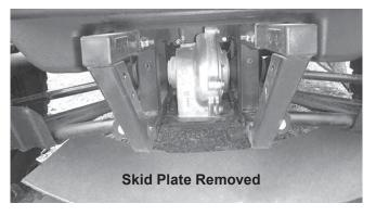
5. Place the skid plate assembly up against the vehicle frame. Place 3/8" washers on each of the eight 3/8" x 2-1/2" cap screws. Insert the fasteners through the skid plate, vehicle frame, and receiving hitch (four per side). Secure with 3/8" washers and 3/8" locknuts; hand tighten.
