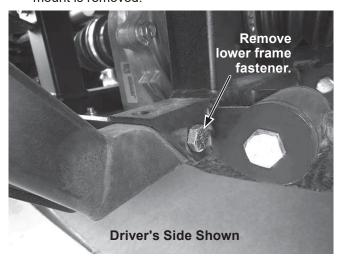
Remove the four fasteners holding the front skid plate in place. Save fasteners for reinstallation if mount is removed.
