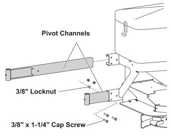
2. Slide the latch channels into the spreader frame on the passenger's side. Install each latch channel to the frame using three 3/8" x 1-1/4" cap screws, 3/8" flat washers, and 3/8" locknuts. Leave the fasteners loose for now.
