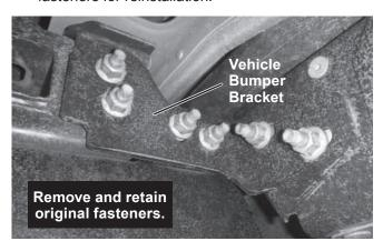
Position the pivot mount driver-side bracket assembly in place of the original bumper bracket. Use the fasteners retained in Step 1 to install the bracket assembly to the vehicle frame and bumper.
