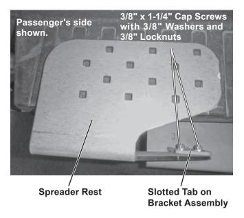
2. Push the spreader rests down until they contact the vehicle bumper. Tighten the spreader rest fasteners according to the torque chart.
