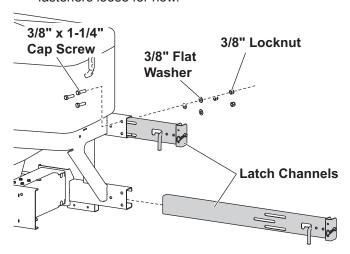
NOTE: The latch channels are slotted to allow for width adjustment of the pivot mount. To ensure a tight channel-to-frame connection, the supplied flat washers must be used with the fasteners installed in these mounting slots.
