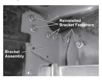
3. Install a 1/2" x 1-1/2" cap screw with 1/2" washer in each of the lower slots of the bracket assembly. Add a second washer and a 1/2" locknut on each cap screw, and hand tighten.
