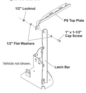
3. Use a level to confirm that the latch bar is vertical. If it is not, shift the top plate forward or backward along the bed rail until the latch bar is vertical. Clamp the top plate in position on the bed rail.
