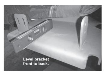
6. Level the passenger-side bracket assembly side to side. Check that the bracket is still level front to back. Hand tighten the fasteners.
