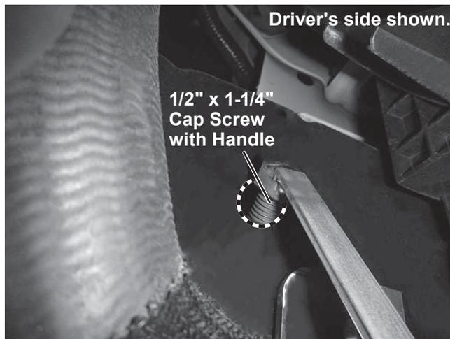
11. Insert a handled 1/2" x 1-1/4" cap screw into the hole found on top of the frame at the front of the vehicle. It may be necessary to trim the handle. Insert the cap screw into the remaining front hole of the mount. Secure with a locknut. Hand tighten the fastener.
