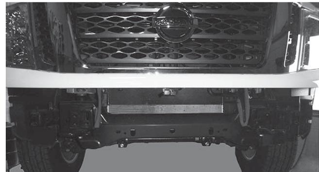
3. Remove and retain the driver-side, passenger-side, and lower plastic radiator shrouds.
