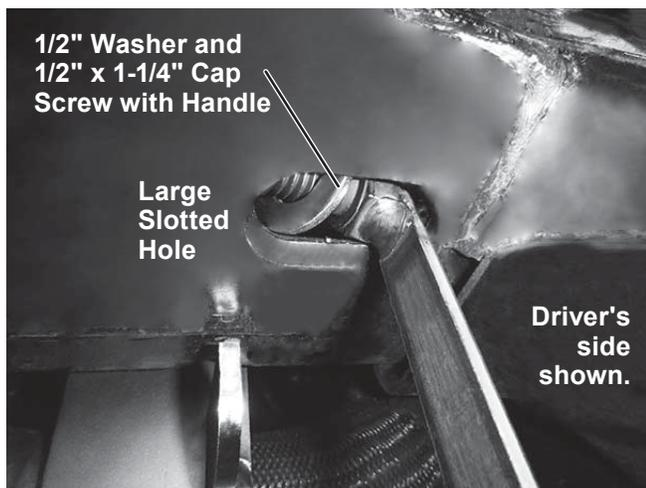
10. Insert a handled 1/2" x 1-1/4" cap screw into the hole found on the inside of the frame behind the radiator. Insert the cap screw in the closest front hole of the mount. Secure with a locknut. Hand tighten the fastener.
