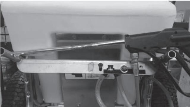
2. Install the handle assembly to the tank base assembly using the provided 5/16" x 1-1/4" cap screws and 5/16" nylon locknuts.
