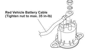
NOTE: Use dielectric grease on all electrical connections to prevent corrosion. Fill receptacles and lightly coat ring terminals before assembly.
