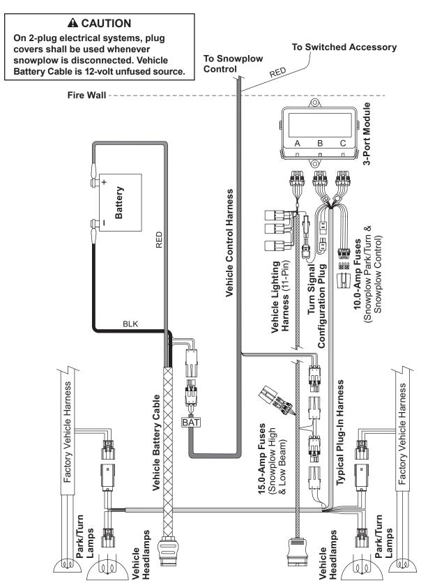
TYPICAL 3-PLUG, 3-PORT MODULE SYSTEM DIAGRAM
