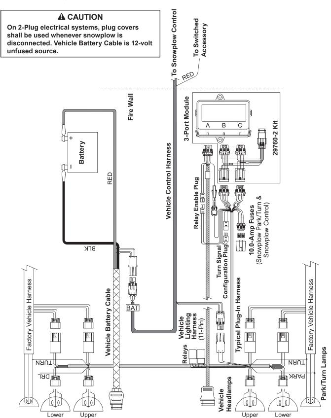
TYPICAL 3-PLUG, 3-PORT MODULE SYSTEM DIAGRAM
