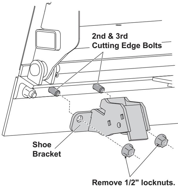
3. Insert the 1/2" x 1-1/2" carriage bolts through the mounting holes in the shoe bracket and install the 1/2" locknuts from the bolt bag. Torque fasteners to 105 ft-lb.
