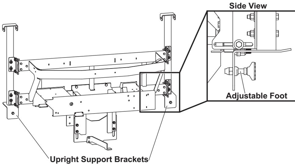
5. Insert the receiver mount into the vehicle's 2" receiver. Lock into place with the hitch pin and cotter.
