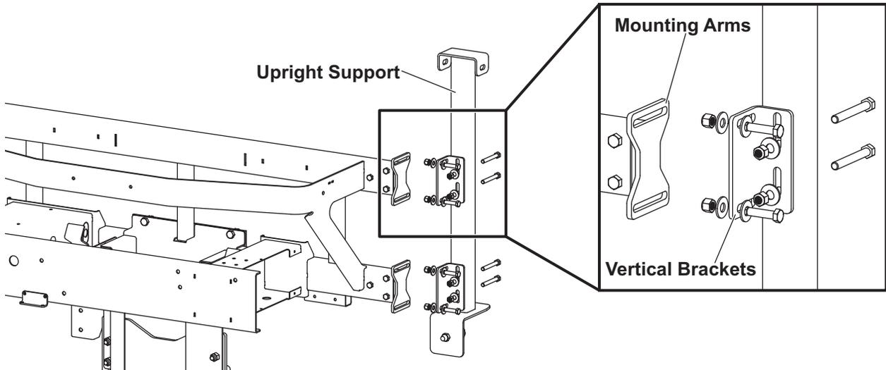
3. Attach the mounting arms to the spreader frame using the supplied hardware.
