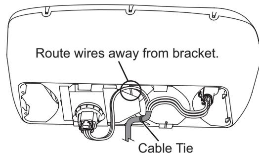
3. Install a cable tie to securely hold the braided portion of the harness against the headlamp. Route the wires where they will not chafe on the steel bracket.
