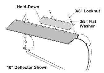
Install one 3/8" flat washer and 3/8" locknut on top of the outermost cap screw and hand tighten. Repeat for the second cap screw. 6. Place a second hold-down over the deflector, with the innermost cap screw through the innermost hold-down hole. The hold-downs may overlap. Install one 3/8" flat washer and 3/8" locknut on each cap screw attaching the second hold-down.
