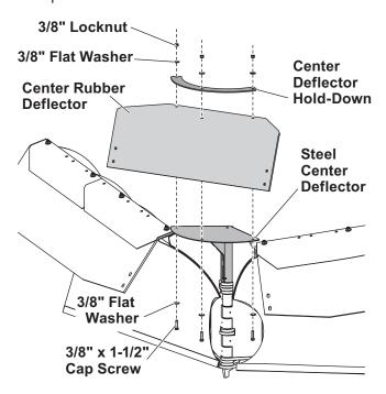
2. Attach the center rubber deflector to the wing rubber deflectors using the provided 3/8" x 1-1/2" cap screws, 3/8" flat washers, and 3/8" locknuts in the pre-made holes.
