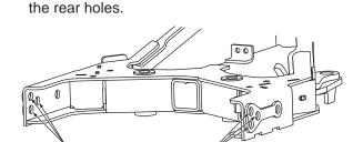
Select the hole in the rear of the T-frame that is aligned closest to the rear holes in the pushbeam.
