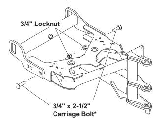
3. Align the rear holes in the pushbeam with the rear holes in the T-Frame and fasten in the middle position using two 3/4" x 2-1/2" carriage bolts\* and 3/4" locknuts. Tighten until assembly is secure, but do not torque at this time.
