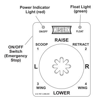
Move the switch on the side of the control to the "ON" position. The power indicator light glows red, indicating the control is ON. The indicator light glows red whenever the control and the vehicle ignition switch are both ON and the electrical connections to the snowplow are completed.
