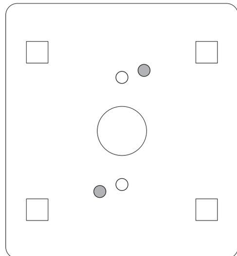
Use this plate and the mounting holes shown for all poly hopper spreader installations.
