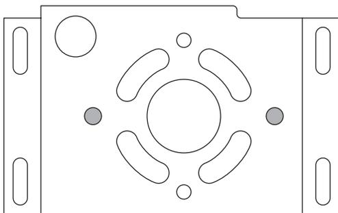
Use this plate and the mounting holes shown for all low-profile tailgate spreader installations.
