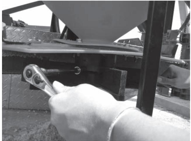
8. Slide the shaft upwards and remove the old spinner.
