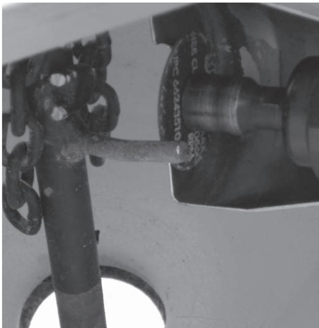
2. Reinstall the locknuts on the upper bearing flange fasteners.
