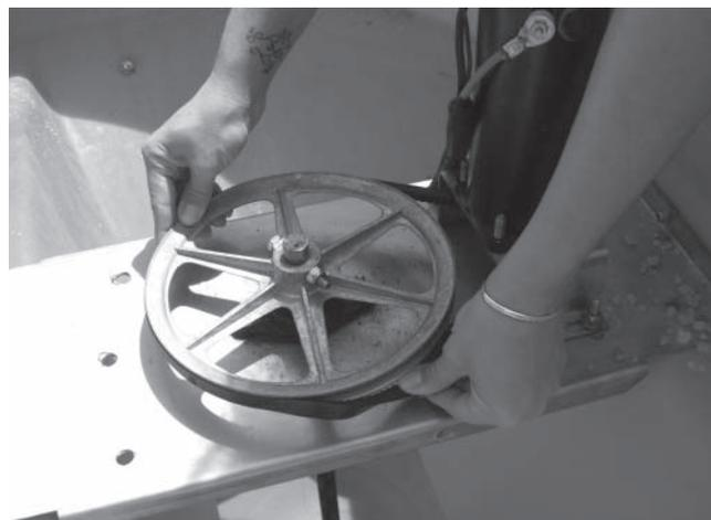
5. Remove the locknuts from the bearing flange fasteners. (Leave set screws tight.)
