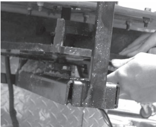
7. Remove the fastener holding the spinner in place.
