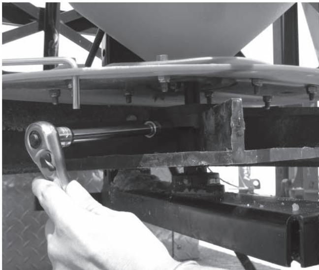
4. Reinstall the belt on the drive and spinner pulleys.
