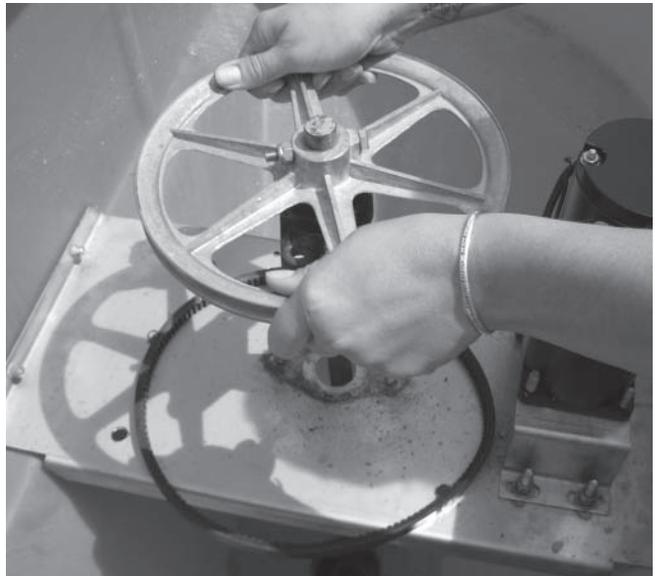
9. Return the old spinner with the deflector rod according to directions received in the service bulletin.
