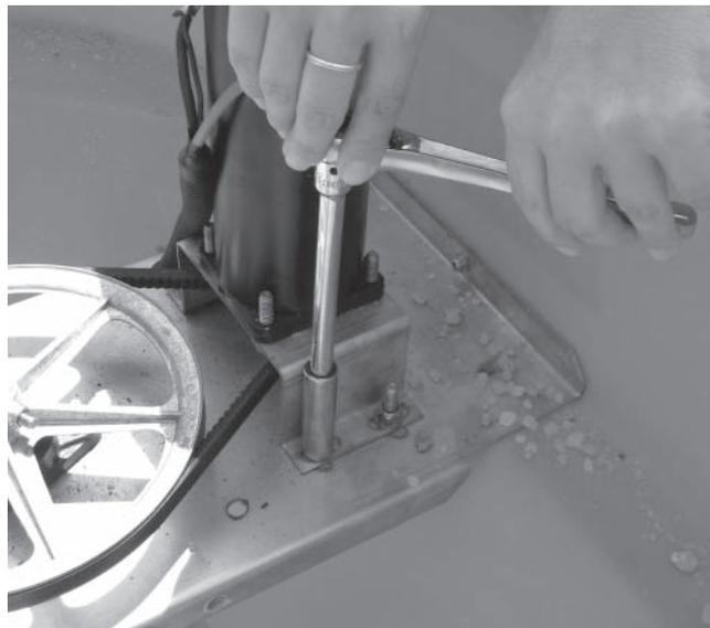
4. Remove the belt from both the drive and spinner pulleys.
