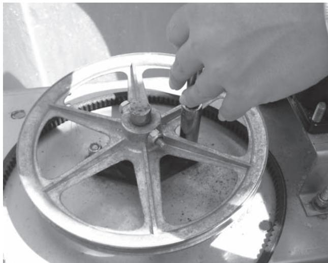
3. Apply medium-strength threadlocker and tighten the set screws on the lower bearing.
