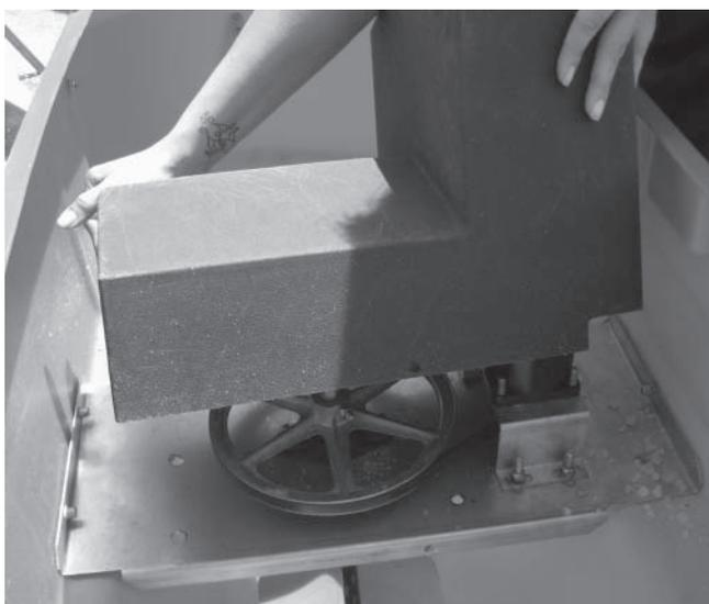
3. Loosen the motor mount fasteners to relieve belt tension.
