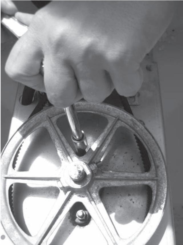
6. Loosen the set screws on the lower bearing.
