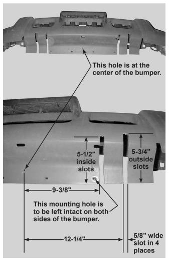
24. Reinstall the front bumper. The bumper wraps under the cross tube of the mount, and the slots in the bottom of the bumper fit around the side plates. The center section of the air dam is mounted with the bumper using the original fasteners.
