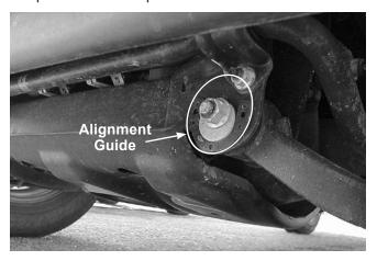
7. Using a punch and hammer remove the two tabs located at the lower rear corners of the mount.
