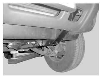
25. The end pieces of the air dam are fastened to both the bumper and the plastic wheel-well using two plastic rivets as shown. This procedure requires the use of a Marson brand Klik-Loc™ plastic rivet setter number 48000 or equivalent, which is available from many local automotive centers or dealerships.
