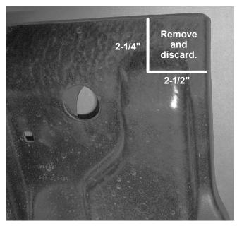
6. On 2002 model year vehicles, inspect the frontend cross member for an alignment guide. If vehicle does not have this guide, skip Step 7 and proceed with Step 8.
