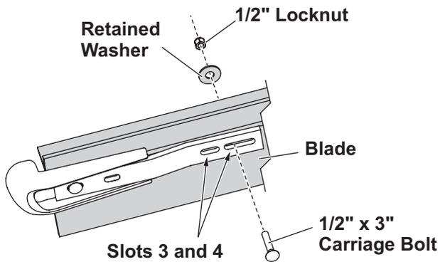
5. Slide the curb guard inward until it is tight against the end of the blade.
