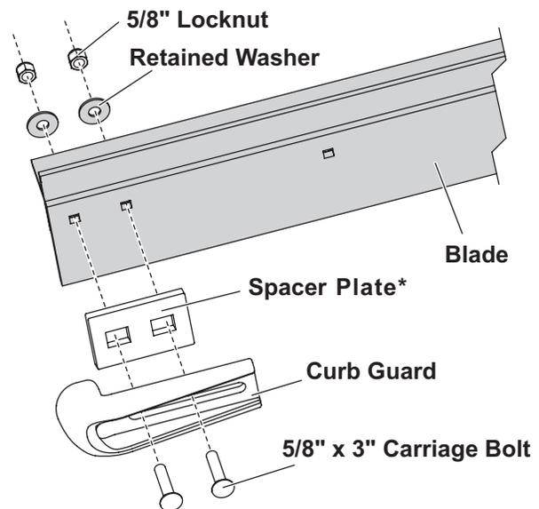
\* For installations where cutting edges include welded-on curb guards.
