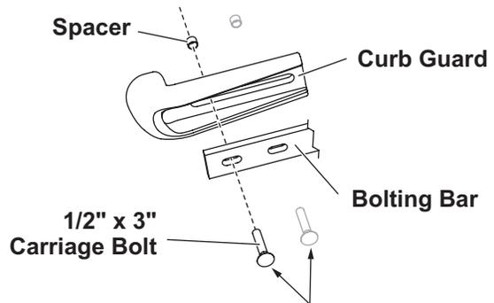
One bolt and spacer for full-length bolting bar.
