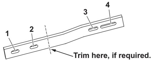
2. If using a trimmed bolting bar: Insert a 1/2" x 3" carriage bolt at *both* slots 1 and 2 on the bar.
