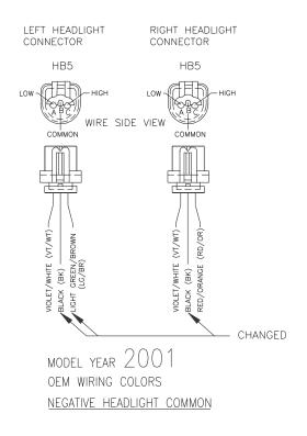
Follow the instructions in the mount box for installing the headlamp plug-in harness. Make the connections to the four headlamp relays as shown in the diagram included with this kit. Revision 3 and later plug-in harness 63413 has a dark blue wire terminated with a fully insulated blade (male) that is not used in this installation.
