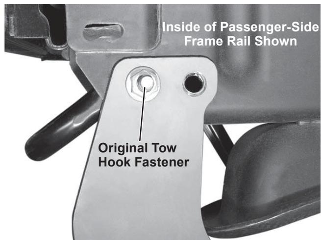
2. Rotate the passenger-side mount plate back, and push it tight up against the bottom of the frame. Clamp the mount plate in place against the frame.
