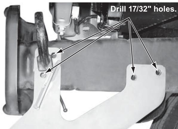
4. Insert two 1/2" x 1-1/2" cap screws with handles and 1/2" flat washers into the inside of the truck frame and out through the rear drilled holes. Attach a 1/2" locknut to each cap screw, and hand tighten.
