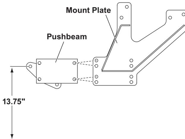
9. Attach the pushbeam to the mount plates using eight 1/2" x 1-1/2" cap screws. Place a 1/2" locknut on each cap screw, and fully tighten according to the torque chart.
