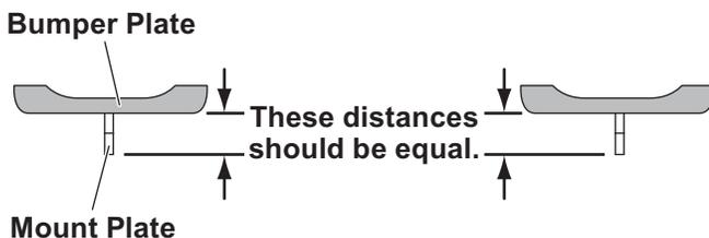
8. Align the four holes in each side of the pushbeam with the holes in the mount plates. Measure the distance between pushbeam and ground, as shown below, to choose which set of holes to use for installing the pushbeam. Choose the set of holes that will bring the pushbeam closest to the dimension shown.
