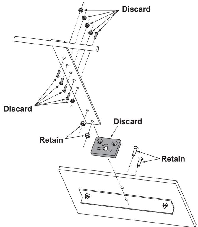
4. Remove the feed gate handle from the feed gate. Retain fasteners.
