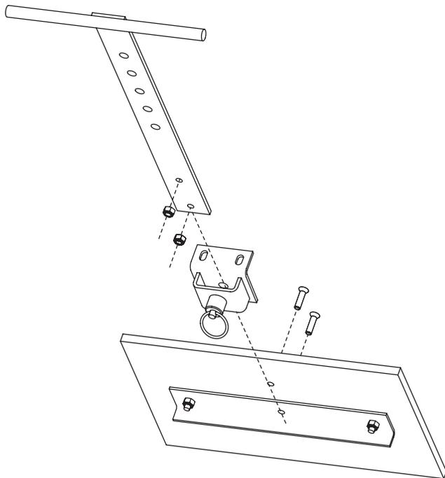
3. Reinstall the feed gate handle onto the feed gate using the original fasteners.
