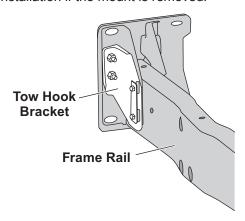
3. Install the mount by holding the front portion of the mount in place and securing with the previously removed bumper bracket bolt assembly. Clamp the rear portion of the mount into position on the truck frame, making sure the mount is tight against the bottom of the frame.
