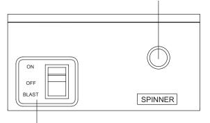
On/Off Control Switch (Emergency stop when required.)
