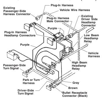
NOTE: All installations of this mount shall have the Park or Turn Harness Kit installed in the plow lights left and right turn signal circuit.
