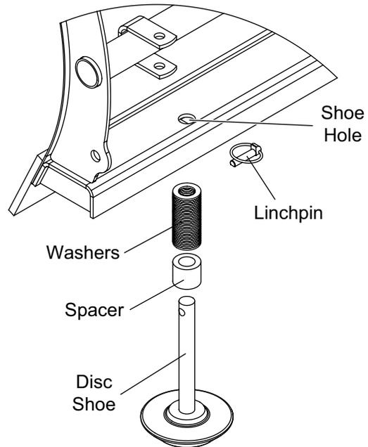
1. Raise the blade 1' off the road surface, turn the control to the OFF position, and from in front of the blade, place jack stands or sturdy blocking under the cutting edge.
