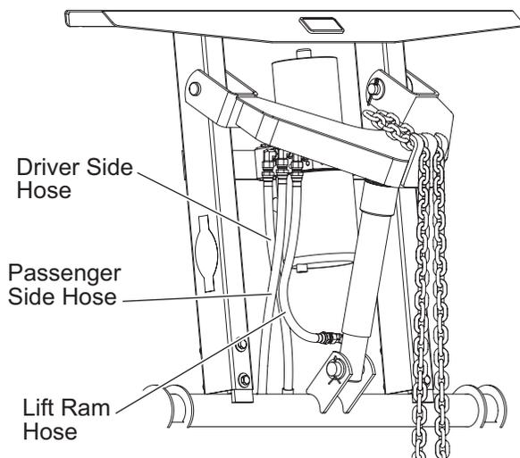
5. Manually angle the blade fully in each direction to remove fluid from the angle rams. Do not allow the hose from the extending ram to take fluid back in.
