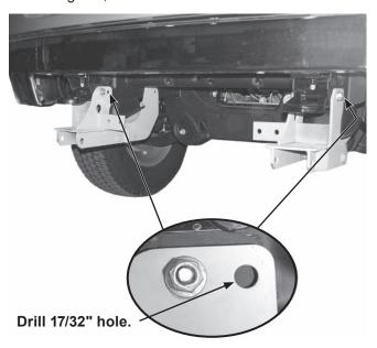
Using the rear holes in the passenger-side mount as a guide, drill two 17/32" holes into the truck frame.
