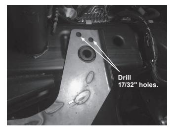
Insert two 1/2" x 1-1/2" cap screws with handles and 1/2" flat washers into the inside of the truck frame and out through the rear drilled holes. Attach a 1/2" locknut to each cap screw and hand tighten.
