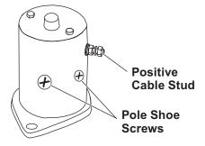
Accurately locate the midpoint between the two pole shoe screws. (Failure to be at the midpoint could result in drilling into the field windings, ruining the motor.)
