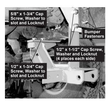
3. Align the large holes and, from the outside of the frame, insert a 5/8" x 1-3/4" cap screw, two flat washers and a locknut on each side of the vehicle. Install a flat washer against the mount frame side plate and against vehicle frame. Depending on vehicle model and year, the hole location for the 5/8" and 1/2" fasteners may vary. Install one fastener for each frame hole.
