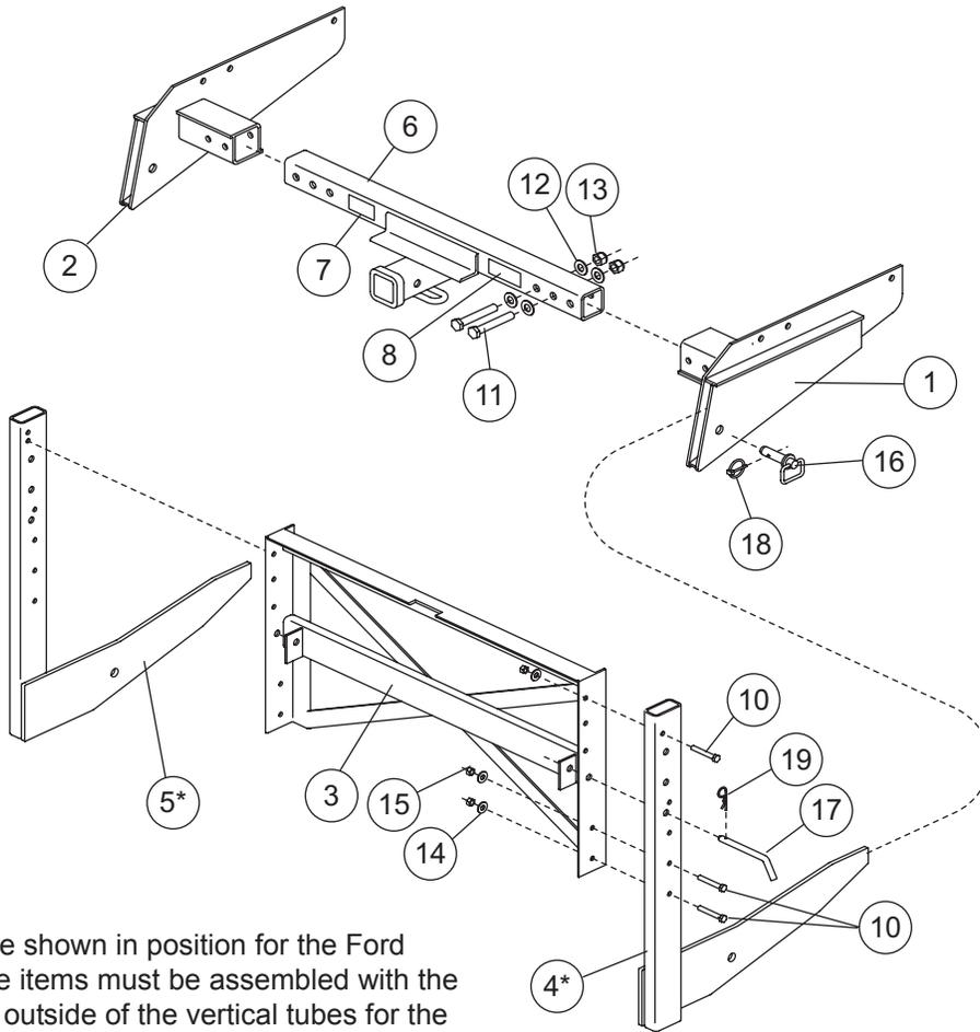
\* Items 4 and 5 are shown in position for the Ford assemblies. These items must be assembled with the mount bars to the outside of the vertical tubes for the Chevrolet/GMC and Dodge assembly. See Figure Below.
